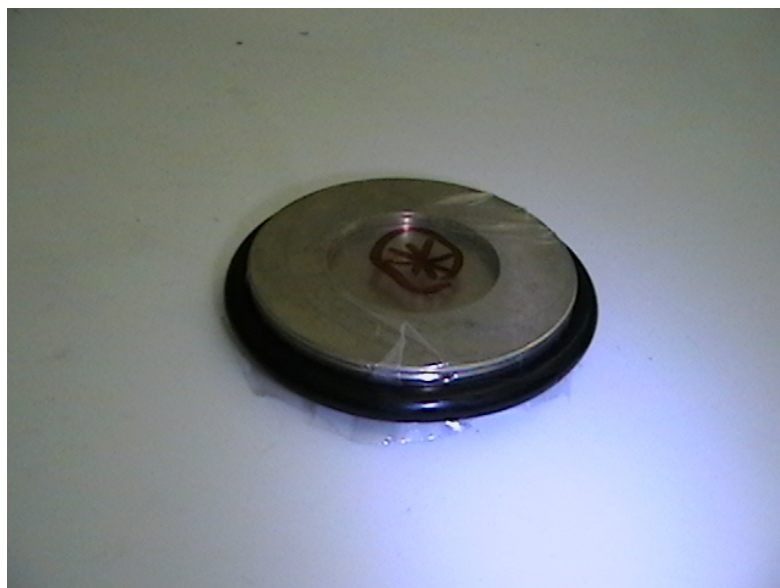
Figure 3.3: XRD Sample Holder Covered with Polyethylene Clear Plastic Wrap.
