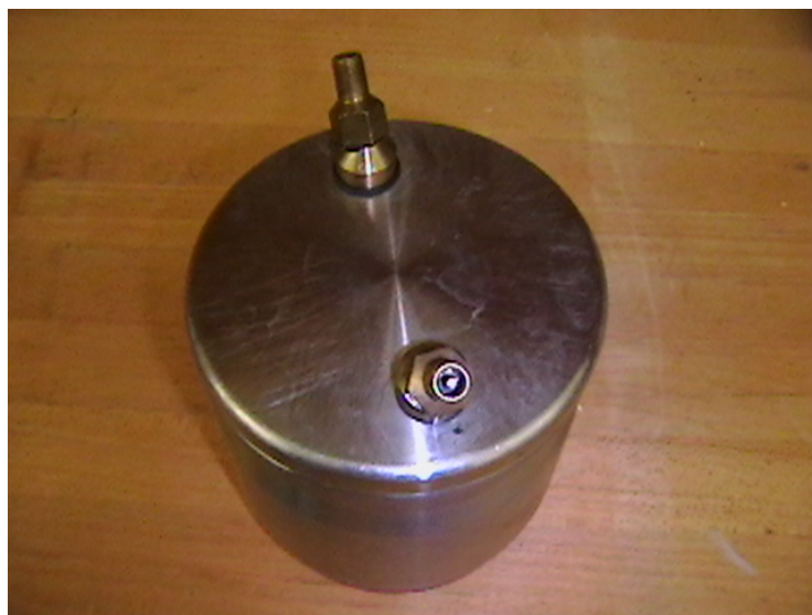
Figure 3.2: Ball Milling Bowl and the Specially Designed Lid with Schrader Valves.
