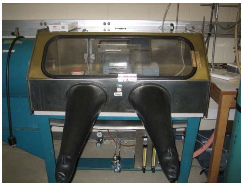
Figure 3.13: SDT-Q600 Inside an Inert Atmosphere Glove Box.
