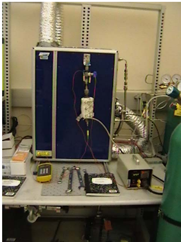
Figure 3.18: PCTPro-2000 Hydrogen Sorption Apparatus Picture.
